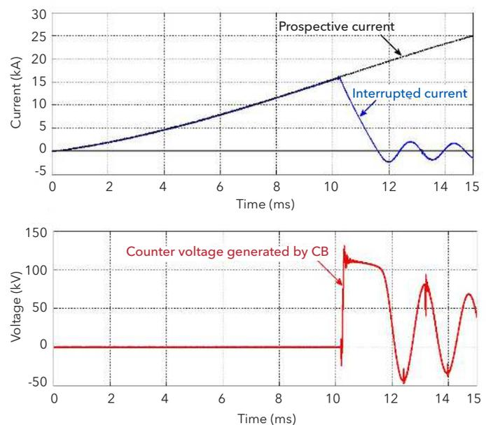
Figure 1 - Test results of active current injection HVDC circuit breaker at KEMA Laboratories
