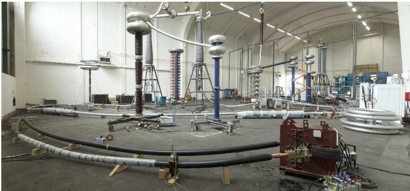
Two unique test requirements in testing a HVDC cable system compared to that of a HVAC cable system exist: a specified maximum temperature drop across the insulation of a cable and a superimposed impulse withstand test.
