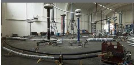
An extended type test program, in accordance with a client's specification, on a 320 kV HVDC cable system, manufactured by General Cable France, has been successfully completed. The test program surpasses the test program of Cigré TB 496. The photograph shows the test set-up for the superimposed voltage tests.
